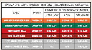
\*Density/Viscosity of liquid used can effect operating range. In very dense liquids, balls may float.
